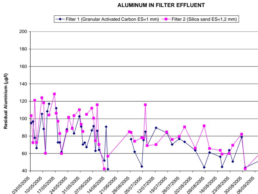
**Chart 2: Analysis of aluminium at the filter effluent**
