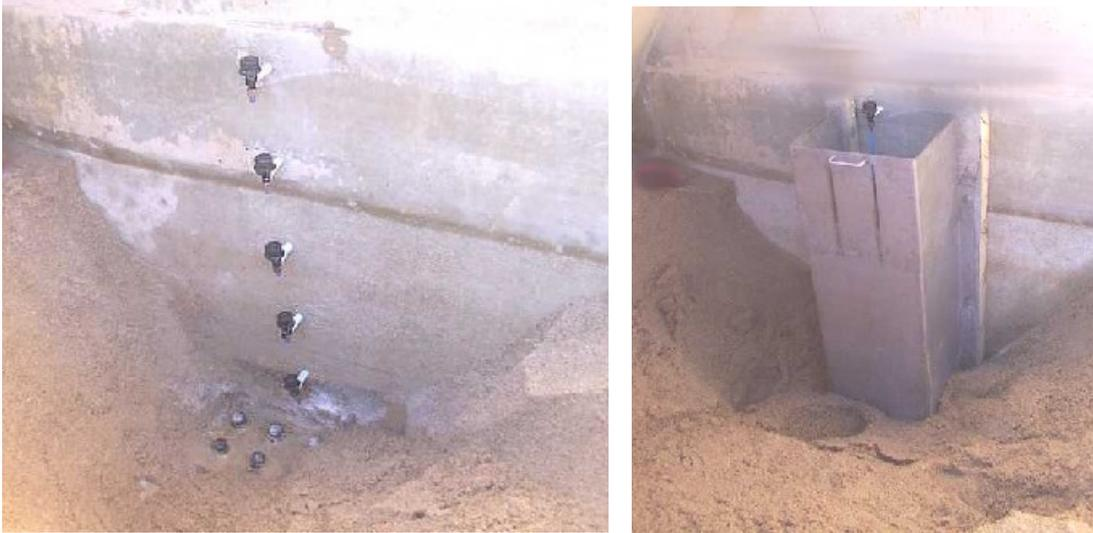
**Photography 1: Pressure drop measurement devices and protection**
