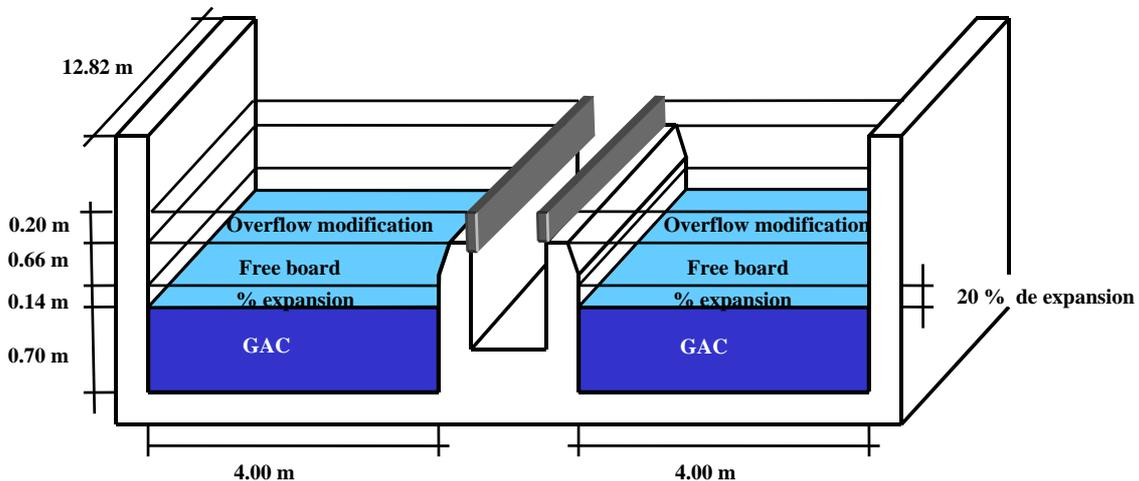
Figure 1: Schematic design modification of the GAC filter
