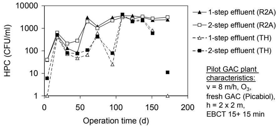
Figure 5. Increase in effluent HPC (R2A or TH, 20 °C, 7 d, pour plate) as a function of time (fresh Picabiol in both columns).
