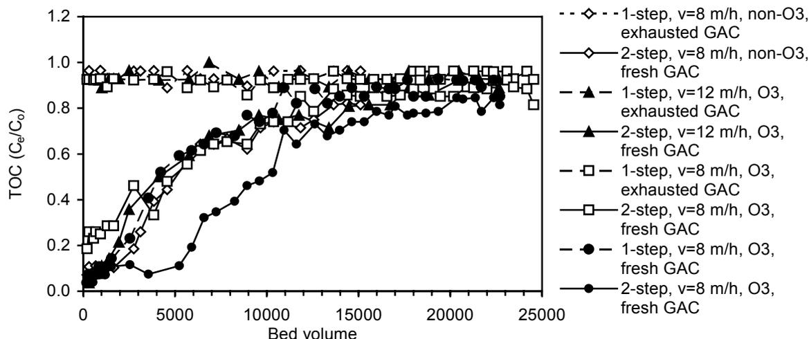
Figure 1. TOC breakthrough curves for two-step GAC filters.
