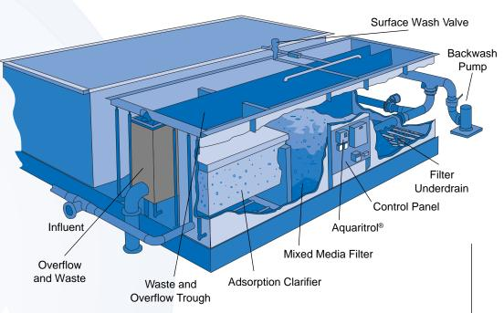
Figure 2: Adsorption Clarifier Package Plant
