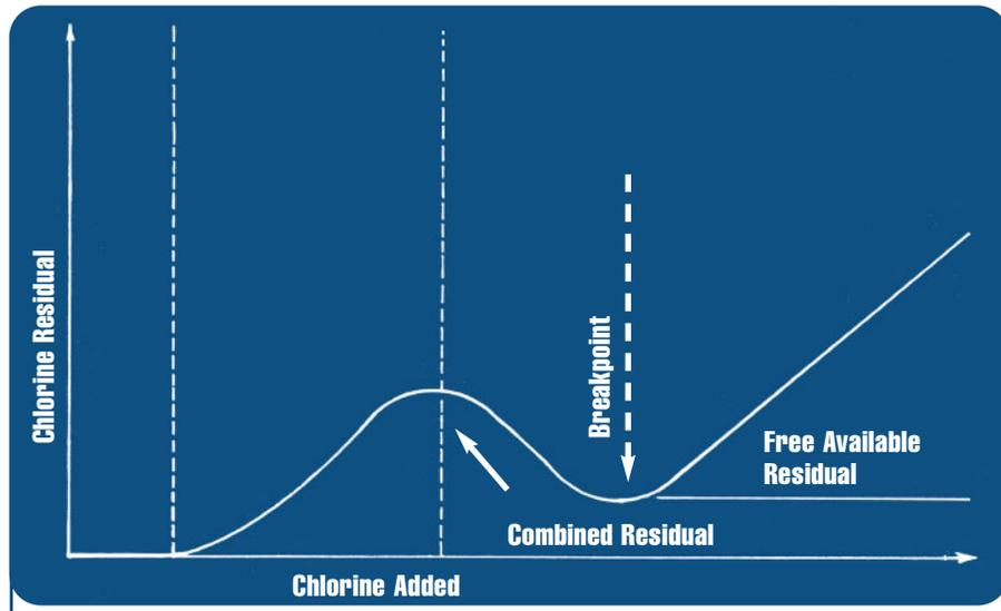
**Figure 1 - Breakpoint Chlorination Curve**
