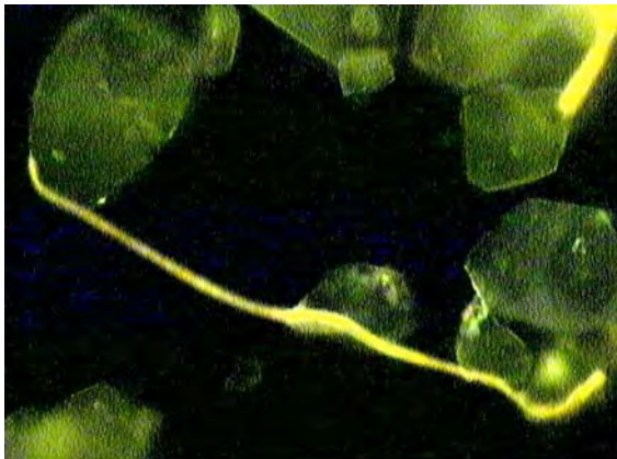
By contrast, water recycled from lime softening sludge lagoon exhibits numerous large, well-formed \text{CaCO}_3 crystals with securely attached or embedded filaments (left); Micrograph (right) shows inclusion of numerous bacterial cells within \text{CaCO}_3 crystals. Absence of planktonic cells indicates that most organisms are particle-associated.
