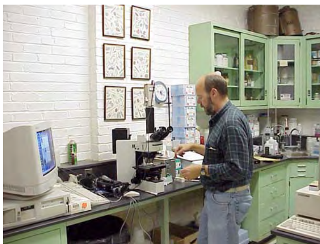
Olympus light microscope with epifluorescence attachment, video camera and computer monitor
